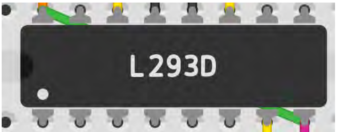
Рис.2.14. H-bridge Motor Driver
